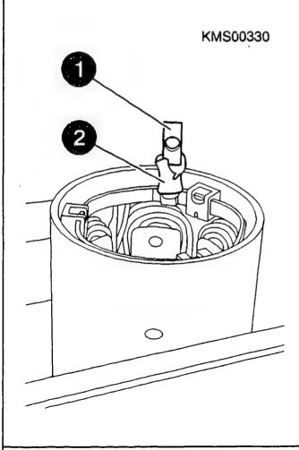
COMPONENT CHECKING AND REPAIR Replacing brush holder Use three-square scraper to remove residual lacquer from stator frame
